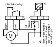
If the digital input is activated, the relay switches on and closes the roller blind. After de-activating the digital input, the relay switches off and opens the roller blind via its N/C-contact.
